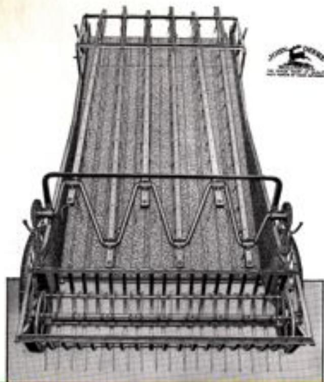
Rear view of loader showing solid steel deck, double-teeth on push-bars, strippers, and other features.
