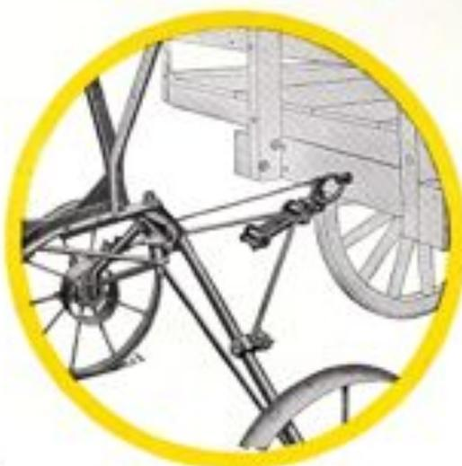
Showing detail of the quick-adjustable hitch on the pivoting foretruck.
