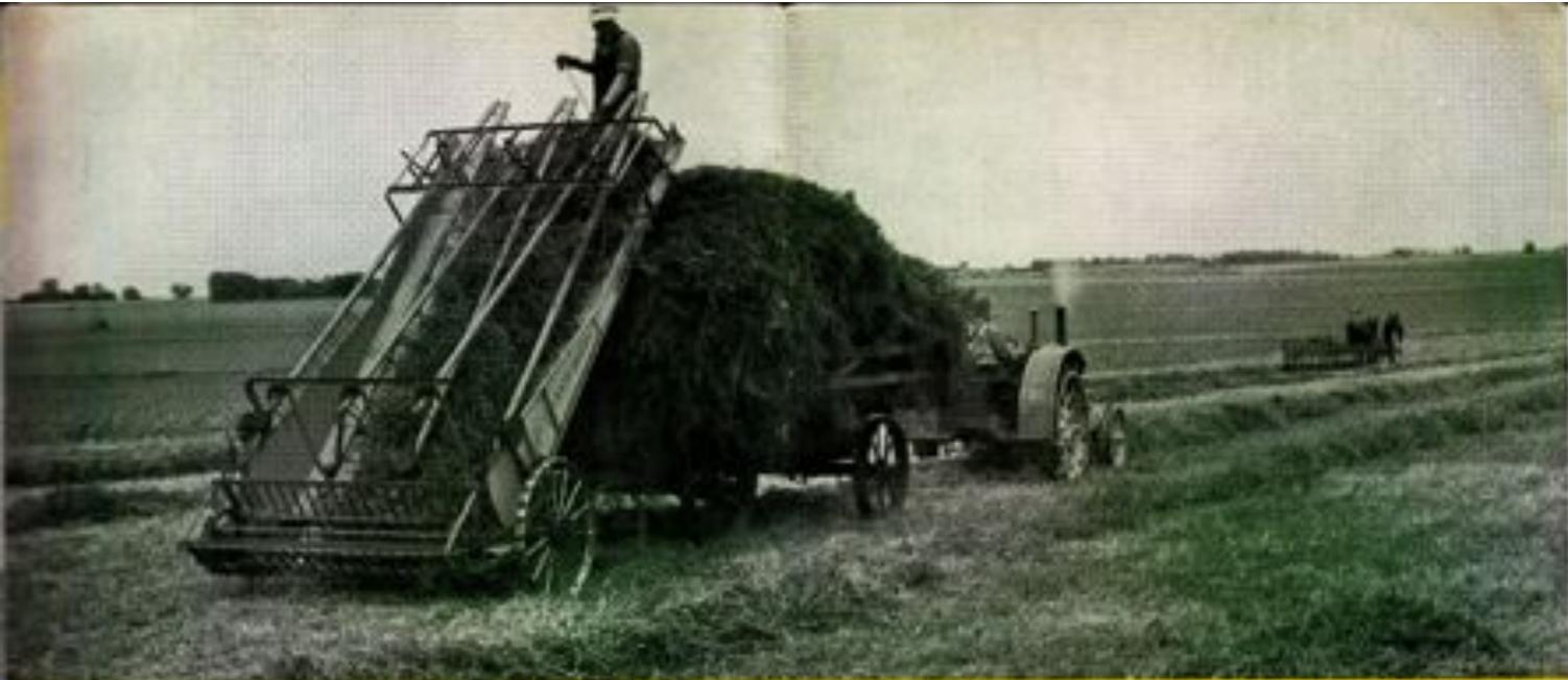
Working with a John Deere Raker Bar-Cylinder Loader in heavy alfalfa.
